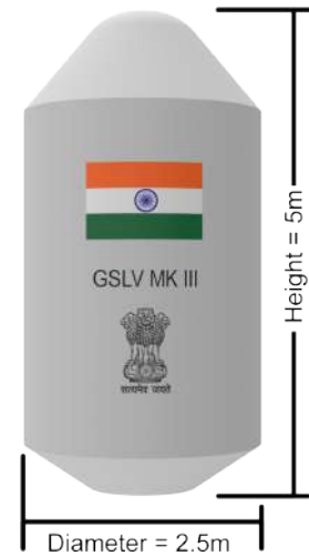
(b) Dimensions of payload fairing
